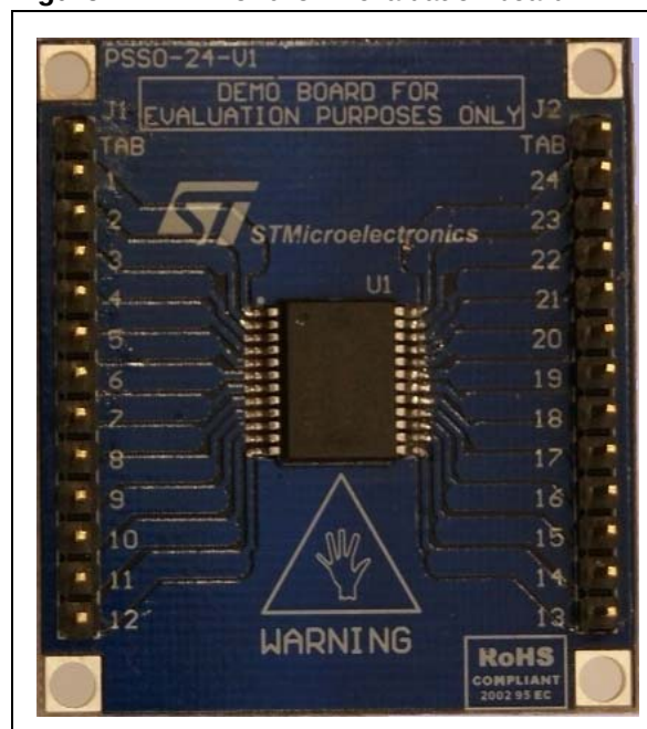
Figure 1. VND5E025AK evaluation board
