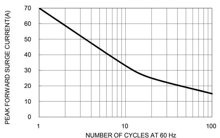
FIG. 2 MAXIMUM FORWARD SURGE CURRENT
