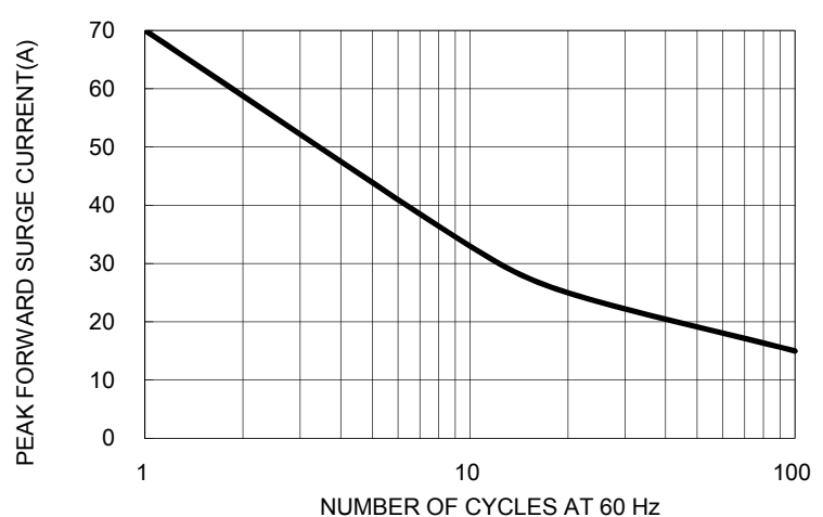
FIG. 2 MAXIMUM FORWARD SURGE CURRENT
