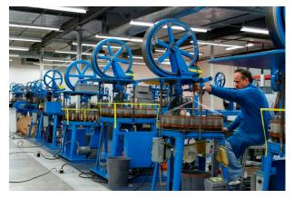
Glenair operates its own high-capacity multispindle overbraiding operation
