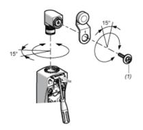
(1) Tightening torque (Min: 1) (Max: 1.5)
