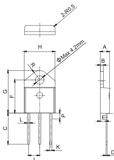
Note: Maximum torque to be applied to mounting tab is 7 in-lbs. (0.8 Nm).
