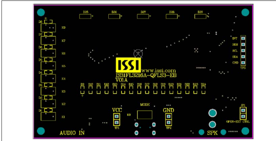
Figure 4: Board Component Placement Guide - Top Layer
