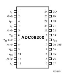
ADC08200 8-Bit, 20 Msps to 200 Msps, Low Power A/D Converter with Internal Sample-and-Hold
