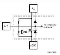
**Note 8:** To guarantee accuracy, it is required that  $V_A$  and  $V_{DR}$  be well bypassed. Each supply pin must be decoupled with separate bypass capacitors. **Note 9:** Typical figures are at  $T_J = 25^{\circ}$ C, and represent most likely parametric norms. Test limits are guaranteed to National's AOQL (Average Outgoing Quality Level).
