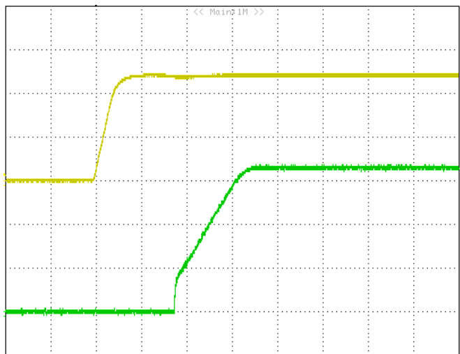
Figure 13: Turn on delay time at 12Vin, 3.3V/20A out. (Green : VOUT, 1V/div, Yellow: VIN, 5V/div. 2mS/div)
