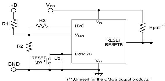
Battery (+B) voltage monitoring: Detects high voltage by R1/R2 resistance dividing.
