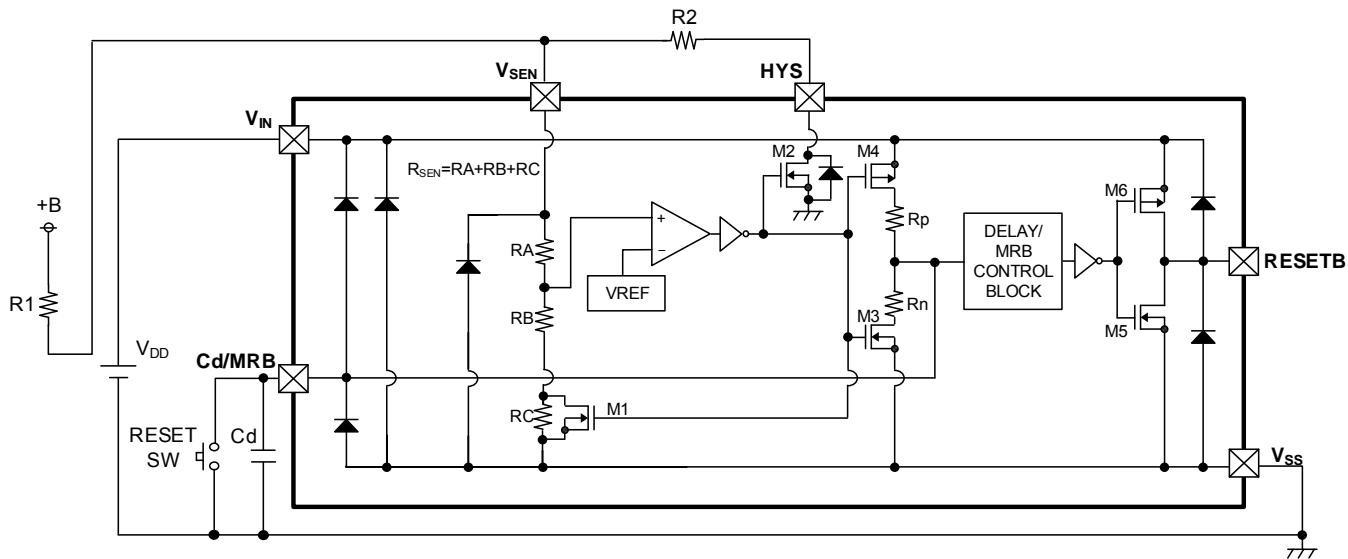
\* The XC6134N series (N-ch open drain output) requires a resistor to pull up the output.
