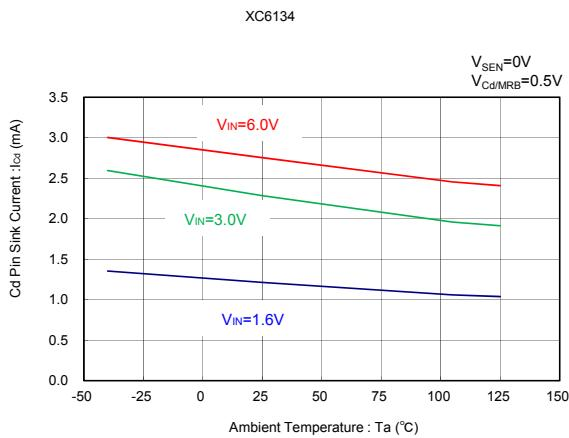
(15) Cd Pin Sink Current vs Input Voltage
