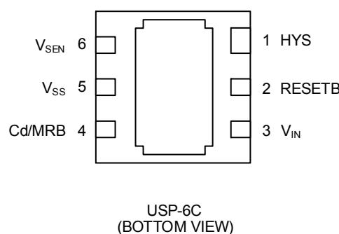
\*The dissipation pad for the USP-6C package should be solder-plated in reference mount pattern and metal masking so as to enhance mounting strength and heat release. If the pad needs to be connected to other pins, it should be connected to V<sub>SS</sub> (No. 5) pin.
