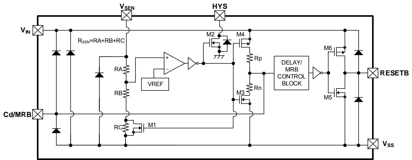
\* Diodes inside the circuit are an ESD protection diode and a parasitic diode.
