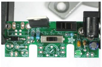
Now we need a way to select which resistor is connected to the regulator. For that we use a 3-way switch. The switch can only go in one way.
