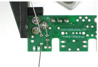
Place one of the 1.0K resistors (Brown Black Red Gold) into the slot marked R1. Then place right next to it one of the 0.1uF ceramic capacitors (they're small and yellow). The resistors and ceramic capacitors are non-polarized so they can go in 'either way'.
