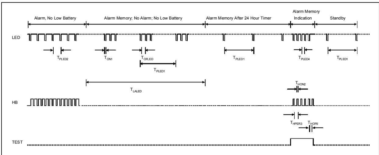
**FIGURE 3-5:** RE46C166/8 Timer Diagram – Alarm Memory Mode.
