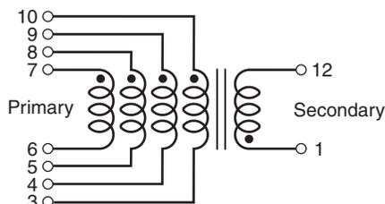
Primary windings to be connected in parallel on PC board
