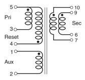
Secondary windings to be connected in parallel on the PC board
