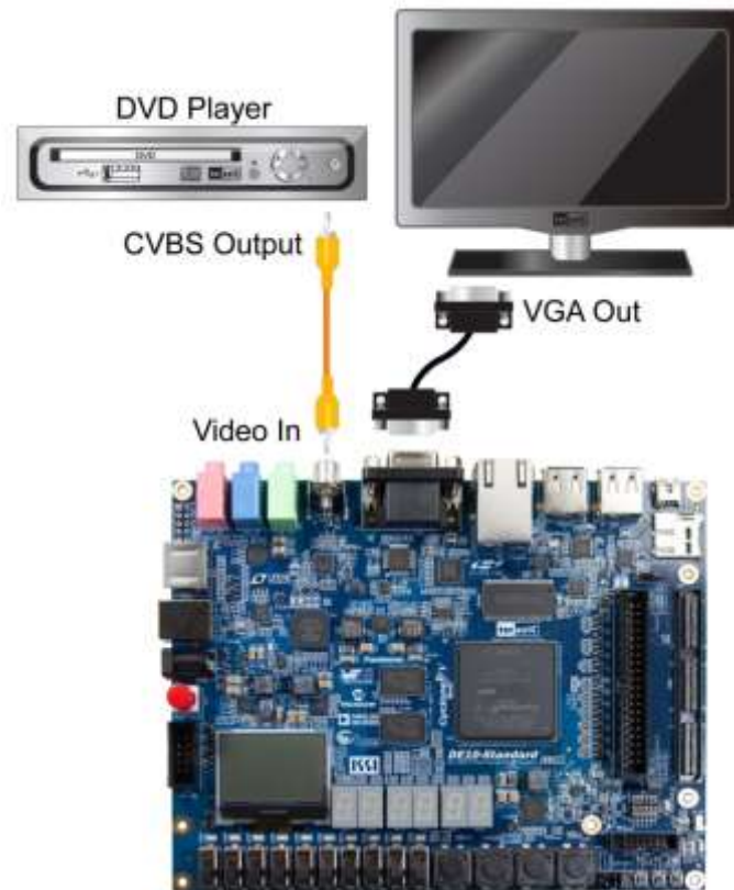
Figure 5-12 Setup for the TV box demonstration (VIP)
