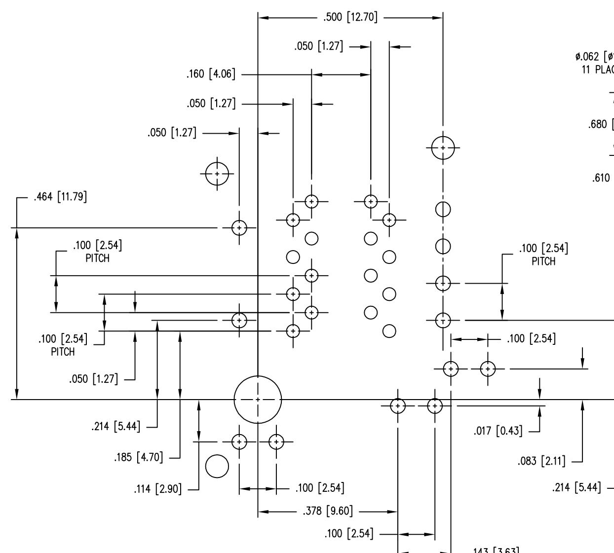
DETAIL A - TYPICAL HOLE LAYOUT
