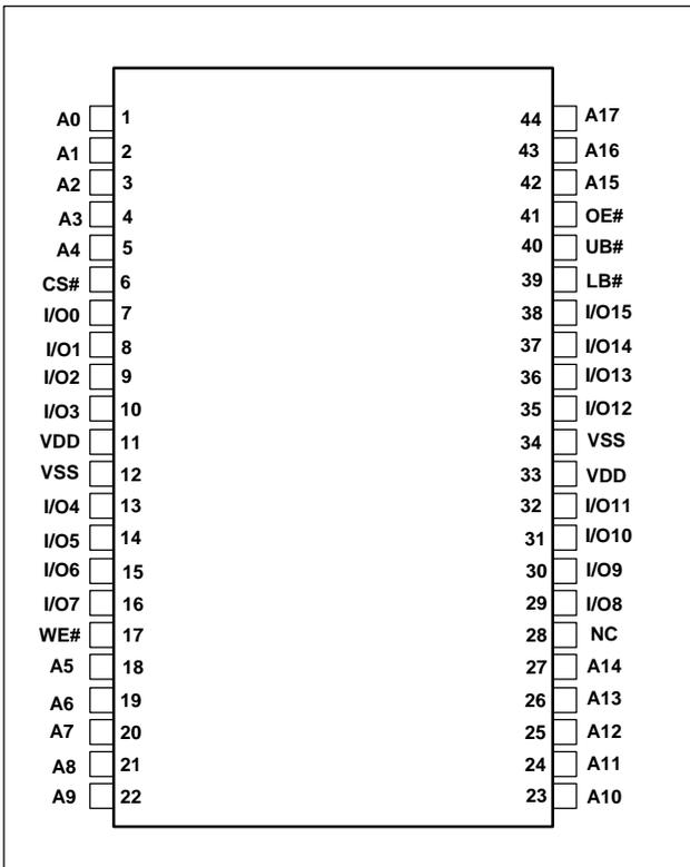
**44-Pin TSOP-II with ERR1, (Package Code : T2)**
