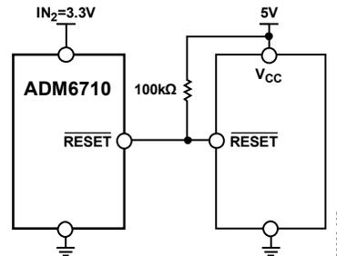
Figure 14. Interface with a Different Logic Supply Voltage
