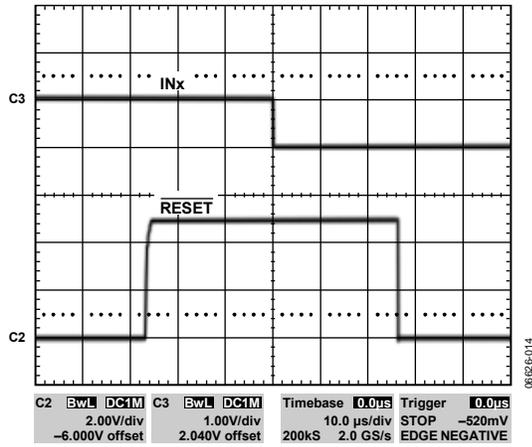
Figure 10. RESET Pull-Up and Pull-Down Response (10 µs/div)
