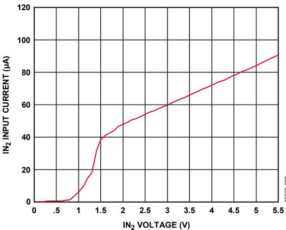
Figure 5.  $IN_2$  Input Current vs.  $IN_2$  Voltage
