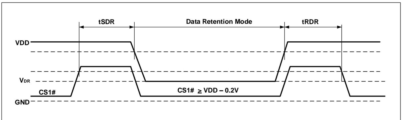
**DATA RETENTION WAVEFORM (CS2 CONTROLLED)**
