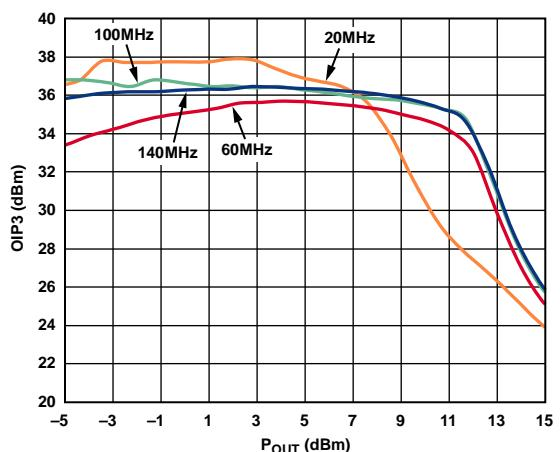
Figure 18. OIP3 vs. Output Power (Pout) and Frequency
