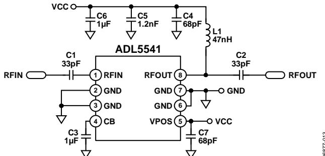
Figure 20. Basic Connections
