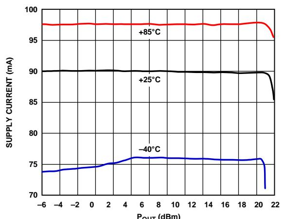
Figure 13. Supply Current vs.  $P_{OUT}$  and Temperature
