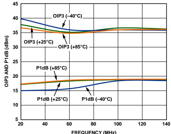
Figure 17. OIP3 and P1dB vs. Frequency and Temperature
