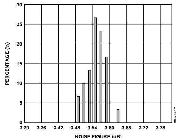
Figure 12. Noise Figure Distribution at 900 MHz
