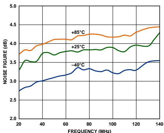
Figure 19. Noise Figure vs. Frequency and Temperature
