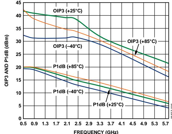
Figure 6. OIP3 and P1dB vs. Frequency and Temperature
