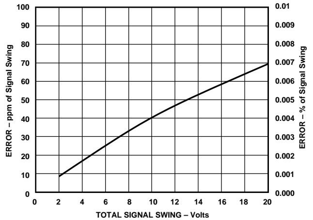
Figure 13. Gain Nonlinearity vs. Output Swing
