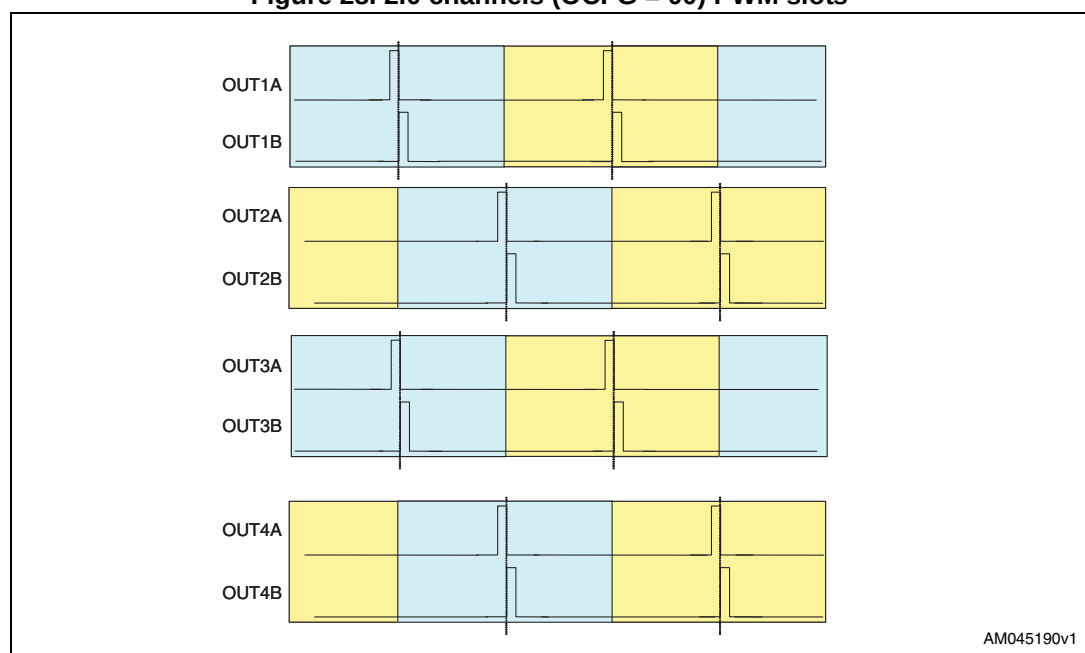
Figure 28. 2.0 channels (OCFG = 00) PWM slots
