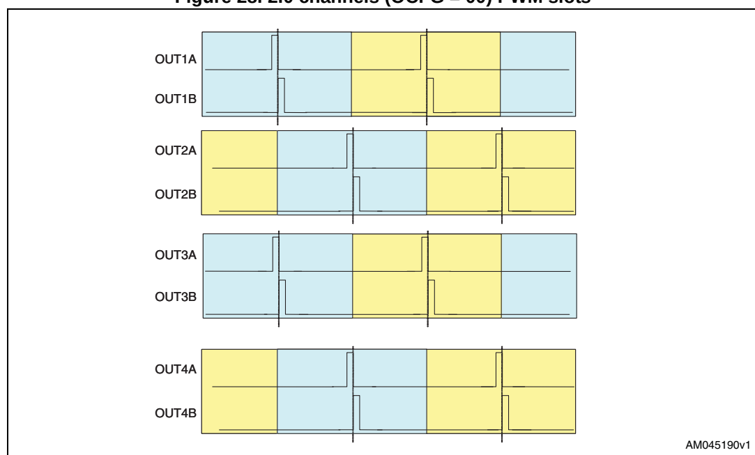
Figure 28. 2.0 channels (OCFG = 00) PWM slots
