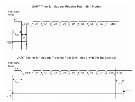
Figure 2. Asynchronous UART Serial Interface Timing Diagram
