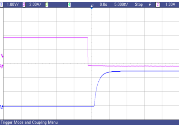
Fig.64 AVO50-48S2V5 typical start-up from CNT on
