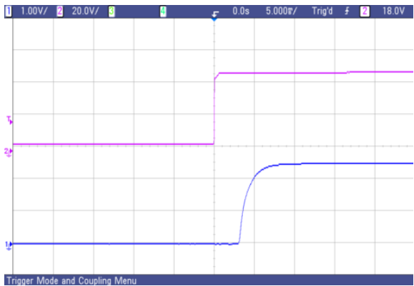
Fig.63 AVO50-48S2V5 typical start-up from power on
