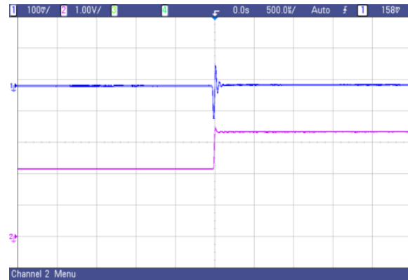
Fig.33 AVO50-48S1V8 typical transient response to step increase in load from 50% to 75% of full load, room temperature, 48Vdc input ( \Delta I_o/\Delta t = 1A/1\mu s )
