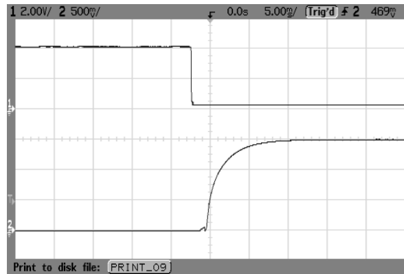
Fig.60 AVO50-48S1V5 typical start-up from CNT on
