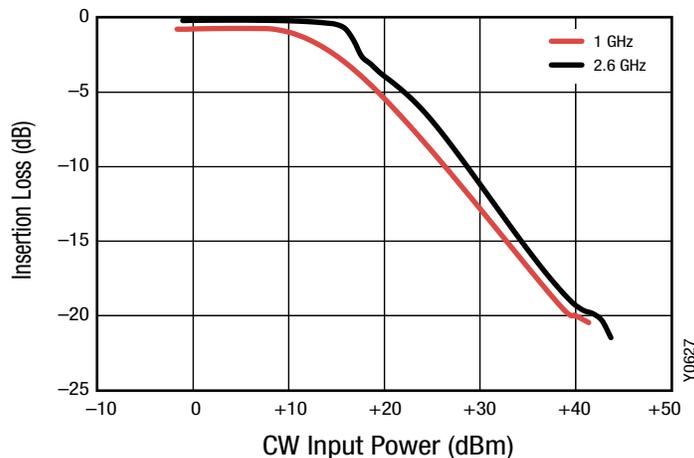
**Figure 4. Insertion Loss vs Input Power**
