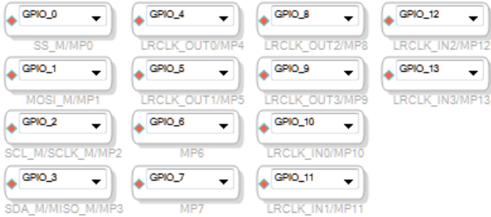
Figure 77. Complete Set of General-Purpose Outputs in SigmaStudio
