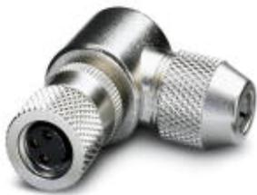
Sensor/actuator connector, socket, angled, 3-pos., M8, shielded, solder connection, metal knurl, cable diameter max. 5 mm
