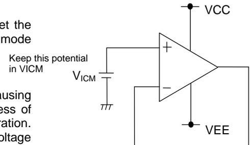
Figure 30. Example of Application Circuit for Unused Op-amp
