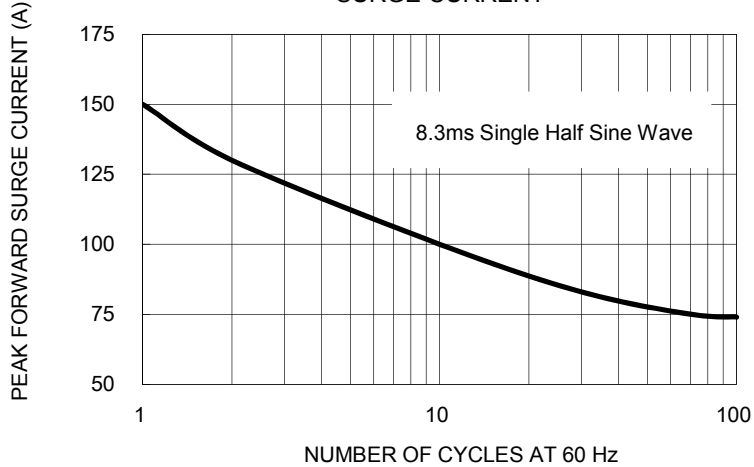
FIG. 3 MAXIMUM NON-REPETITIVE FORWARD SURGE CURRENT
