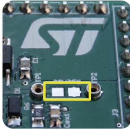
Figure 5. Pads for soldering SMD resistor
