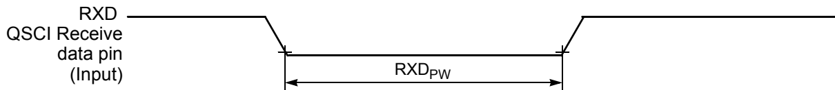
Figure 10-12 RXD Pulse Width
