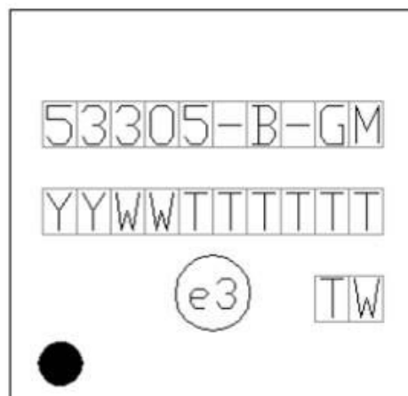
Figure 8.6. Si53305 Top Marking
