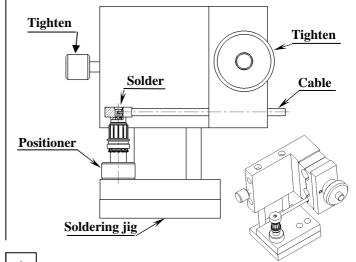
Place cable assembly into a dia D = 6.85 +-0.1 and thickness E = 12.3 +-0.1.
