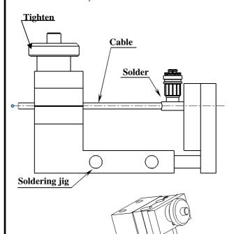
After cooling remove the cable assembly from the jig. Slide the body in position unlocked into the positioner until its bottoms against the positioner. Slide cable assembly into the jig and tighten. Solder the center contact.
