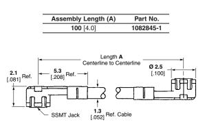
Notes: 1. Consult Tyco Electronics for non-standard cable lengths. Cable length tolerance: Length A Tolerances. Length A Tolerance 50 To 100 [3.94]  $\pm 3 [\pm .12]$ 101 To 500 [3.98 to 19.69]  $\pm 5 [\pm .20]$ Over 500 [19.69]  $\pm 10 [\pm .39]$ 2. To avoid damaging the cable, minimize time at temperature while soldering and/or applying heat to unterminated end of cable.
