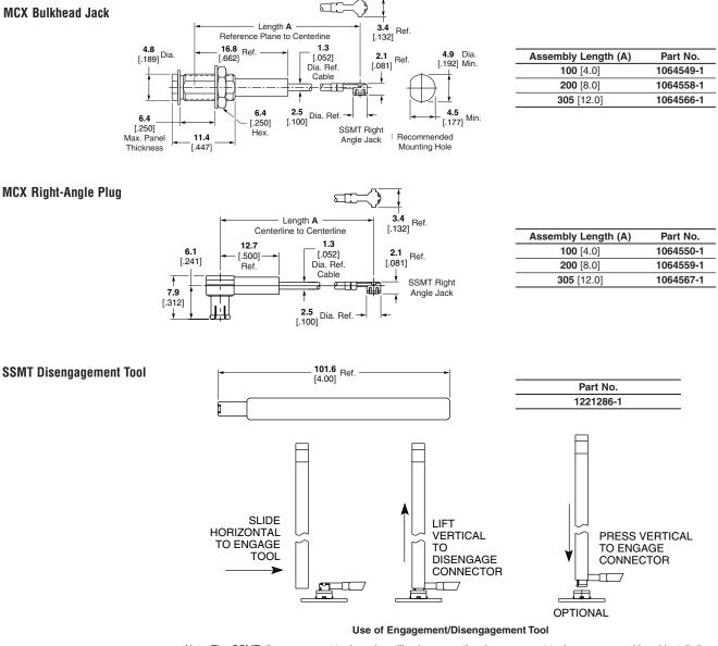
Note: The SSMT disengagement tool can be utilized as an optional engagement tool versus manual hand installation.
