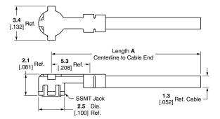
Notes: 1. Consult Tyco Electronics for non-standard cable lengths. Cable length tolerance: Length A Tolerances. Length A Tolerance 50 To 100 [3.94]  $\pm 3 [\pm .12]$ 101 To 500 [3.98 to 19.69]  $\pm 5 [\pm .20]$ Over 500 [19.69]  $\pm 10 [\pm .39]$ 2. To avoid damaging the cable, minimize time at temperature
