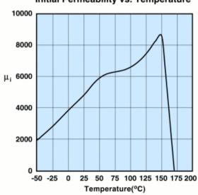
Measured on a 17/10/6mm toroid at 10kHz.
