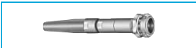
PFG.00 Fixed receptacle, with two nuts, key (G) or key (B), with bend relief (back panel mounting)
