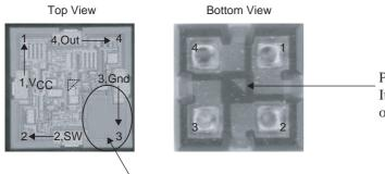
Pin 1 mark It is located at the center of the bottom of the pakage.
