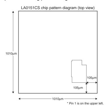
LA0151CS photo-receiving pattern enlarged diagram (effective area)
