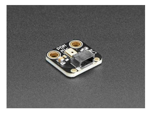
The first thing to note is that this sensor does not provide an 'analog' output like many of our electret microphone
