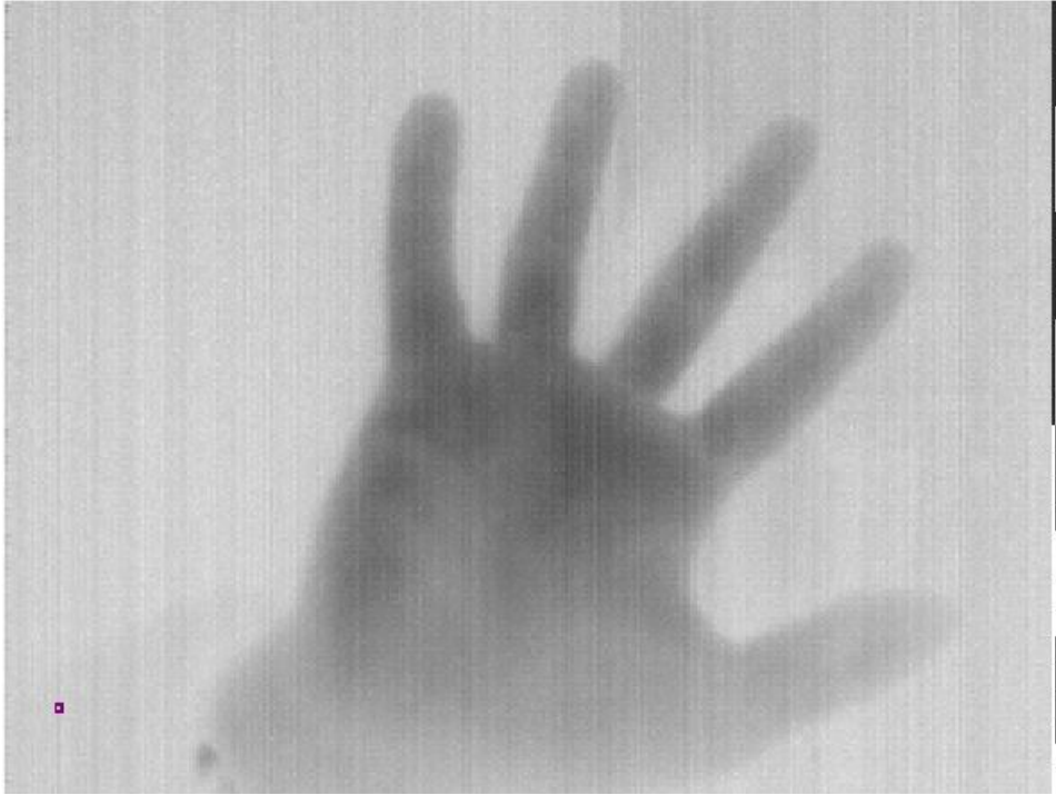
Figure 9: Raw tap A phase0 image of a hand with enabled test columns
