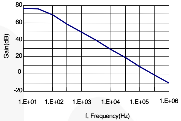
Figure 3. Open-Loop Voltage Gain
