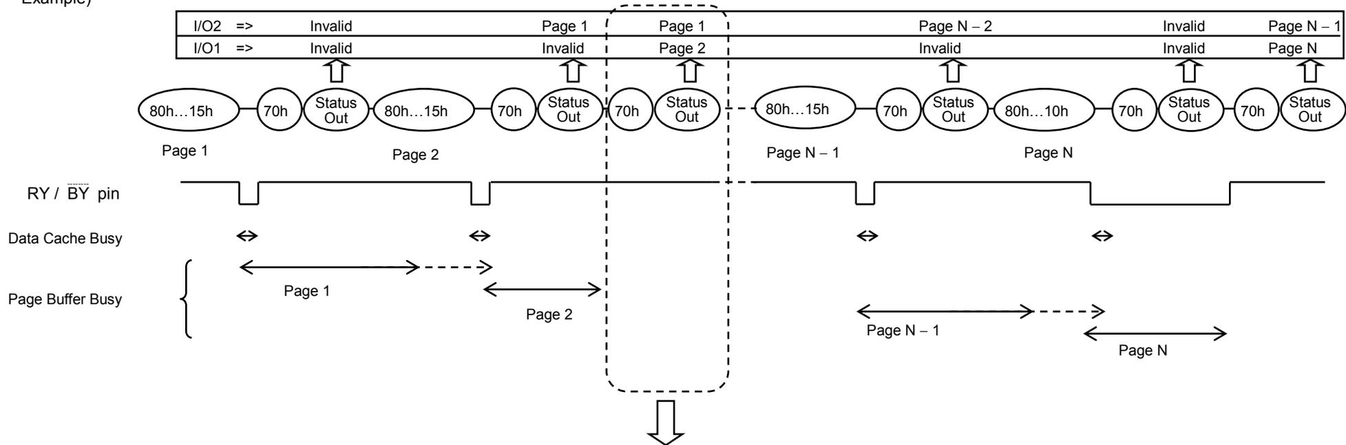
If the Page Buffer Busy returns to Ready before the next 80h command input and Status Read is done during this Ready period, the Status Read provides the Pass/Fail result for Page 2 on I/O1 and the Pass/Fail result for Page 1 on I/O2.
