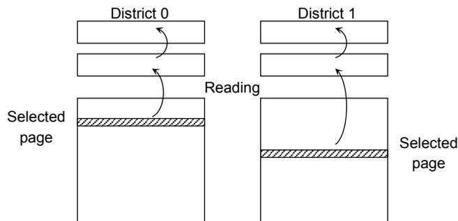
The data transfer operation from the cell array to the Data Cache via Page Buffer starts on the rising edge of  $\overline{WE}$  in the 30h command input cycle (after the 2 Districts' address information has been latched). The device will be in the Busy state during this transfer period.
