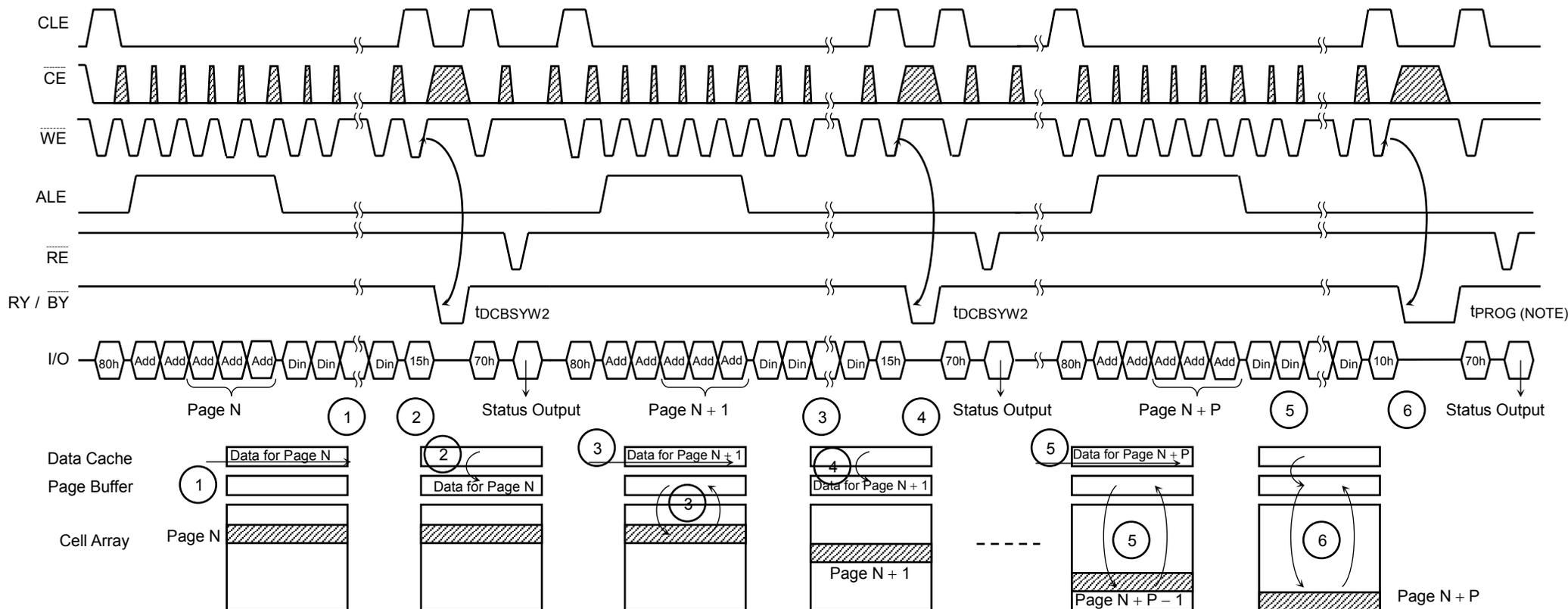
Issuing the 15h command to the device after serial data input initiates the program operation with Data Cache.
