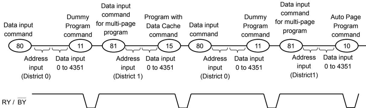
After either “15h” or “10h” Program command is input to the device, physical programming starts as follows. For details about Auto Page Program with Data Cache, refer to “Auto Page Program Operation with Data Cache”.
