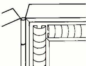
Strips with sticky fingers® are low compression, adhesive mounted Recyclable Clean Copper shielding products. Designed as a continuous band, the strip is slotted to permit spring contact throughout its length. A wide radius profile creates the greatest contact for maximum conductivity with minimum compression requirements.
