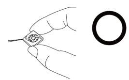
Don't pull fan with lead wires.
