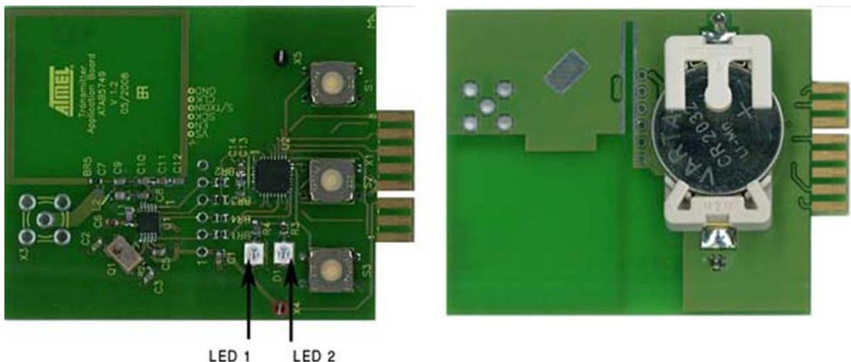
Figure 1-2. Schematic of the Demo Board ATAB5749
