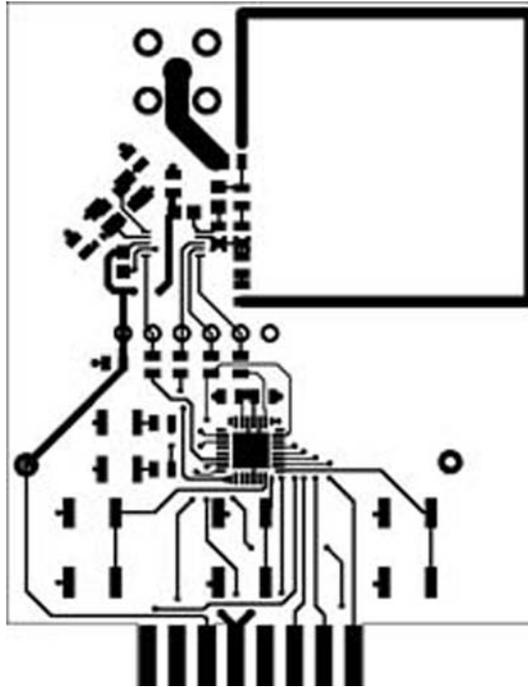
Figure 1-4. Bottom Layer of the Demo Board ATAB5749
