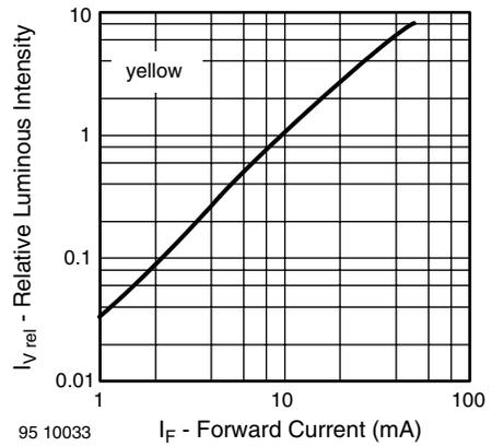
Fig. 11 - Relative Luminous Intensity vs. Forward Current
