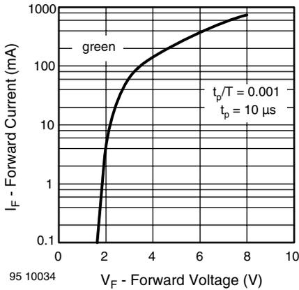
Fig. 13 - Forward Current vs. Forward Voltage
