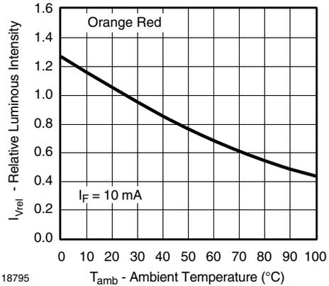
Fig. 4 - Rel. Luminous Intensity vs. Ambient Temperature
