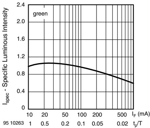
Fig. 15 - Specific Luminous Intensity vs. Forward Current
