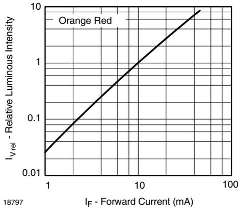
Fig. 6 - Relative Luminous Intensity vs. Forward Current
