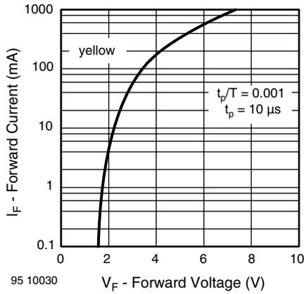
Fig. 8 - Forward Current vs. Forward Voltage
