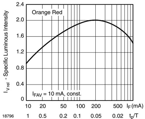
Fig. 5 - Rel. Lumin. Intensity vs. Forw. Current/Duty Cycle
