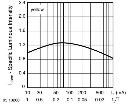
Fig. 10 - Rel. Lumin. Intensity vs. Forw. Current/Duty Cycle
