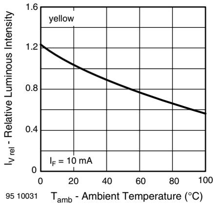
Fig. 9 - Rel. Luminous Intensity vs. Ambient Temperature
