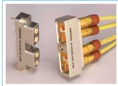
Compliant Pin Quadrax Board Level Connector
