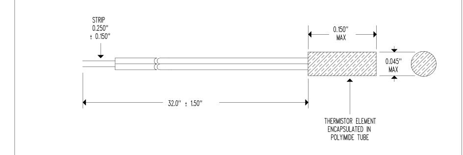
RESISTANCE @  $+25^{\circ}$ C = 10,000  $\Omega$  NOMINAL ACCURACY (+15 TO +80°C) =  $\pm$  0.50°C RESISTANCE/TEMPERATURE CURVE = "J" BETA " $\beta$ " (0 TO +50°C) = 3,892°K NOMINAL TEMPERATURE COEFFICIENT @  $+25^{\circ}$ C = -4.4%/°C NOMINAL MAXIMUM TEMPERATURE RATING =  $+140^{\circ}$ C
