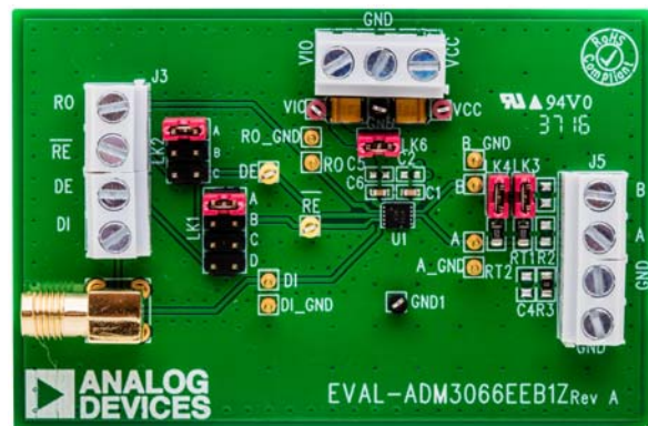
Figure 2. EVAL-ADM3066EEB1Z Evaluation Board
